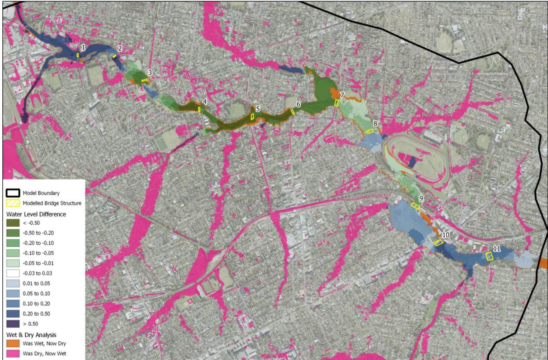
Figure 3-13 Peak Water Level Result Differences (in metres) – 1% AEP Event - Updated Flood Model Less 2009 Mainstream Study Model
