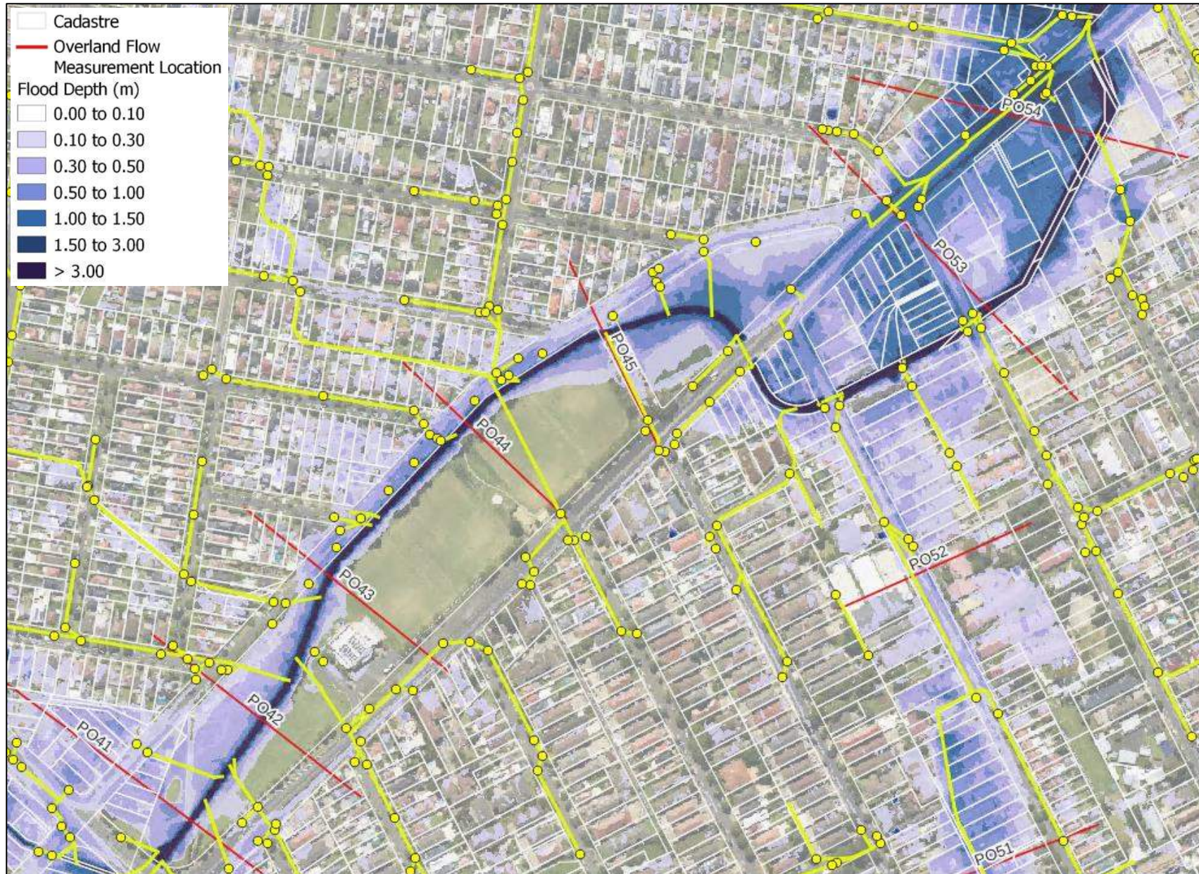
Figure 5-7 Lakemba Local Centre - Flood Mitigation – Parry Park and Coxs Creek (Modelled Pit and Pipe shown in Yellow)
