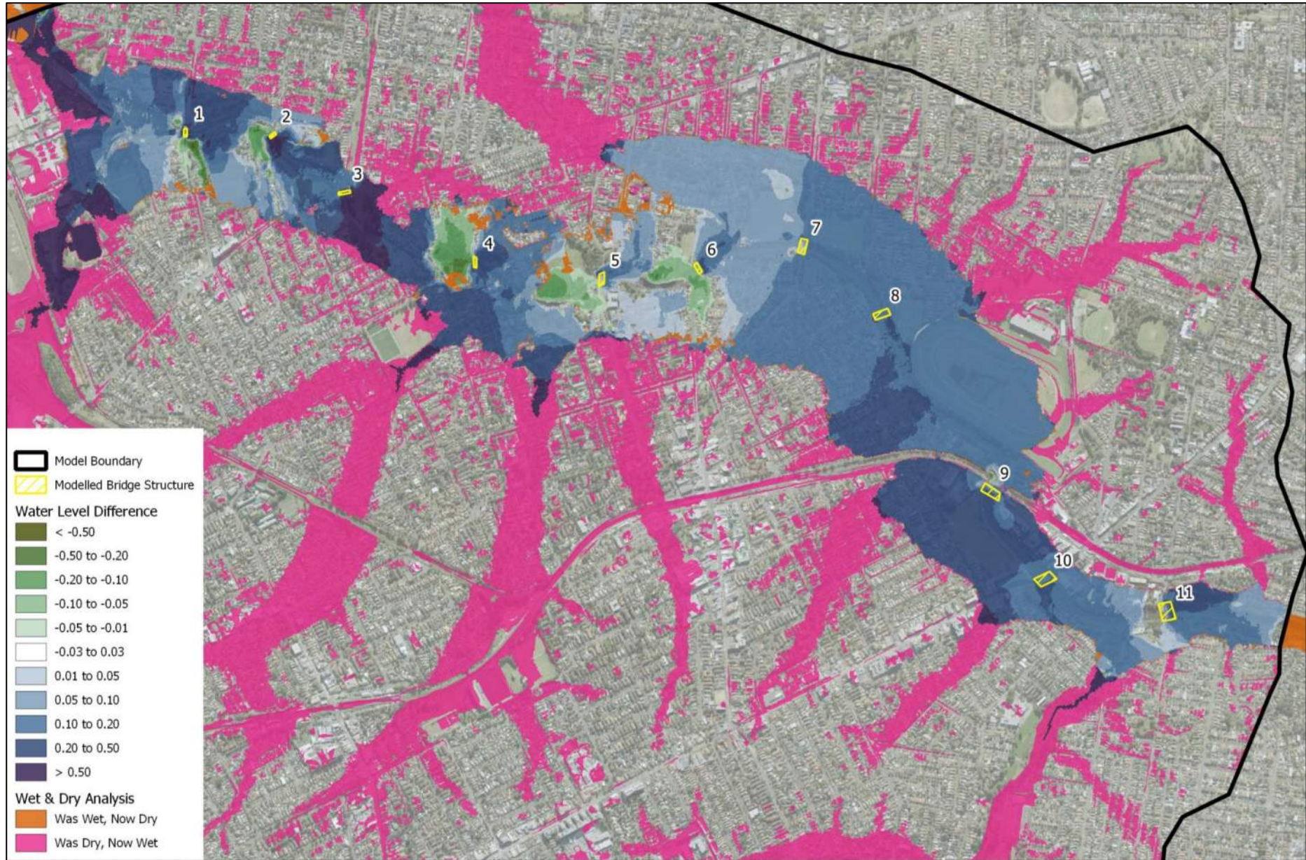
Figure 3-14 Peak Water Level Result Differences (in metres) – PMF Event - Updated Flood Model Less 2009 Mainstream Study Model
