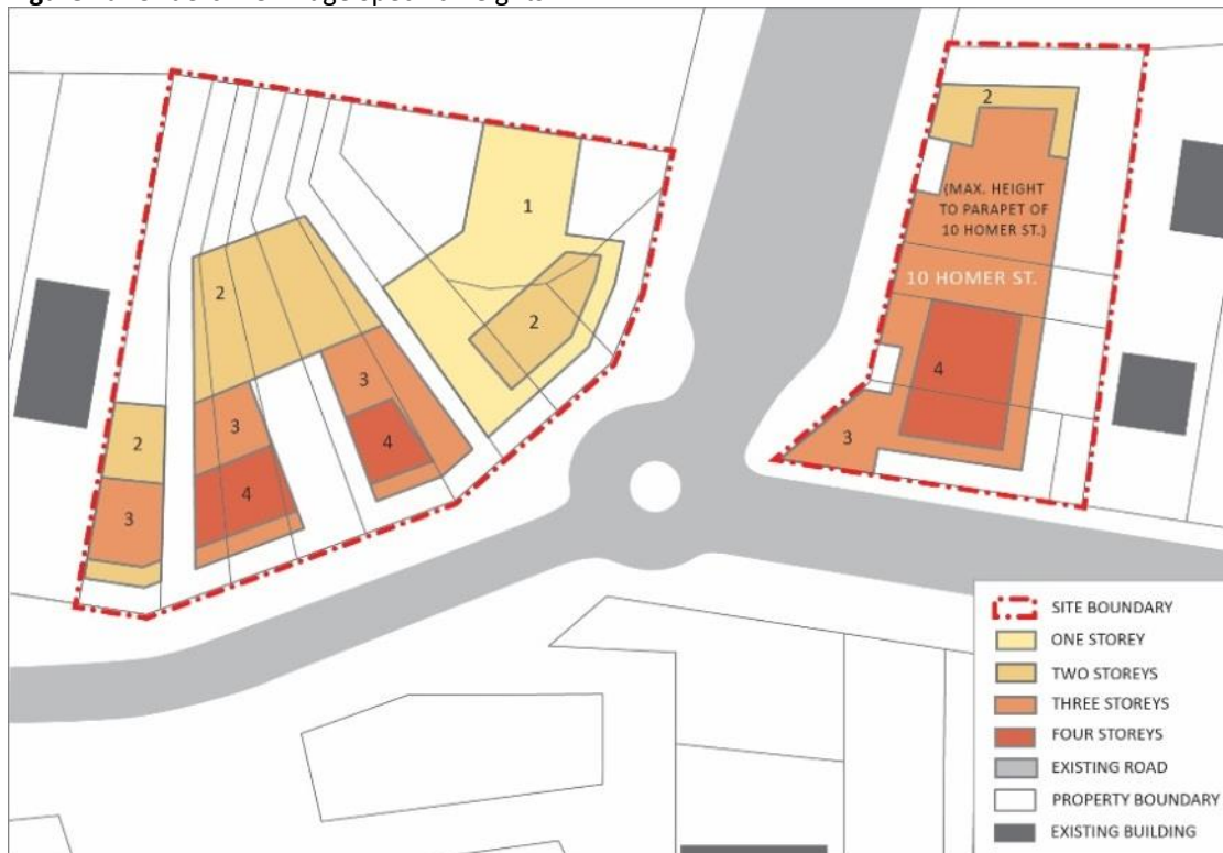
Figure 1a: Undercliffe Bridge Specific Heights
