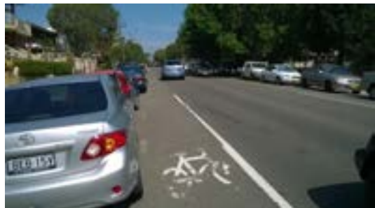
Figure 5.8: Bike Lane in the Door Zone
